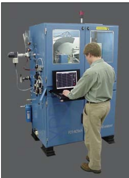
Figure 1. The FCT ACTech COSMA clinker and cement XRD analyser, with operator access. The unit is fully automatic for installation in the plant at the sampling point.
